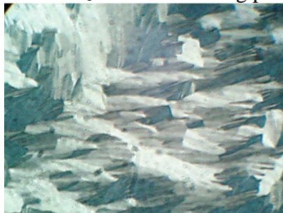
Fig. 5.3. Photomicrograph of solution (SAS 2 35 r. % in water) under the temperature of 23 °C (x 250). Polyline harp texture.
